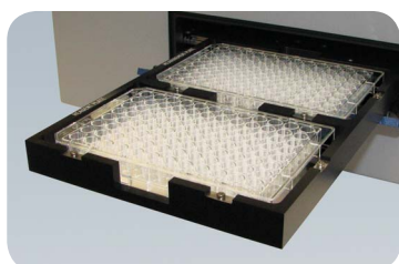
Dual microplate carrier with reagent plate and measurement plate
