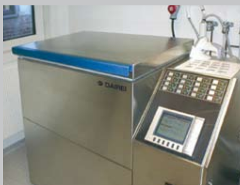
The lid can be opened during freezing process if you need to freeze more blood bags/ampoules
