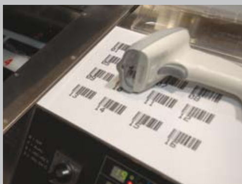
The barcode reader ensures unique logging of the freezing phase of each blood bag/ampoule. It is constructed according to ISP 128.
