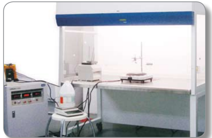
Filter efficiency testing according to BS 7989
