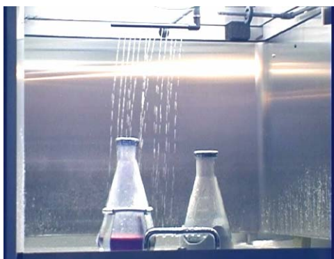
„in a downpour“ Testing the seal
