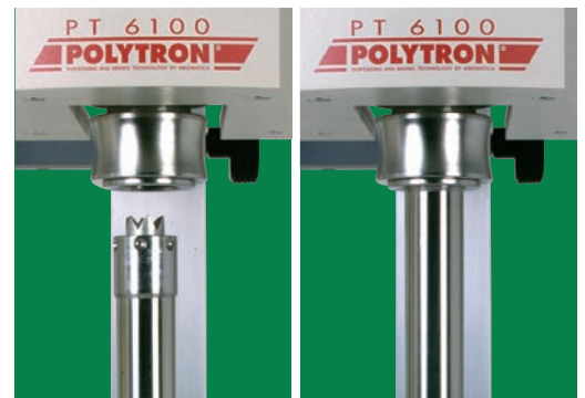
Lock the dispersing aggregate to the drive unit with the safety quick-coupling
