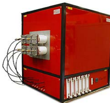
6 Tube sintering furnace with gas tight ends and flow meters
